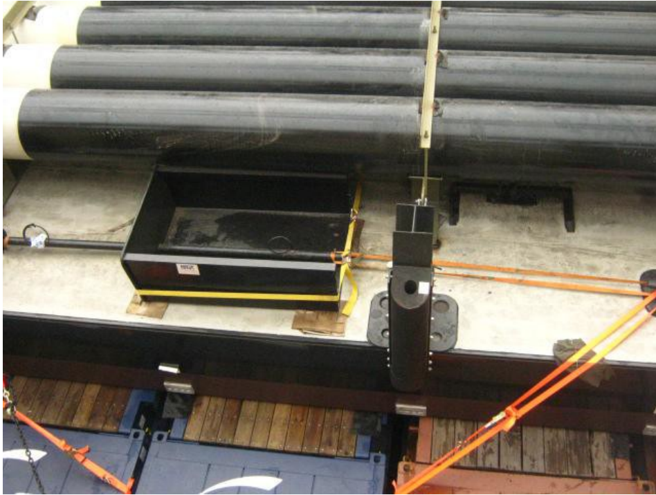
Cargo was properly stowed and secured under deck at bay 58
