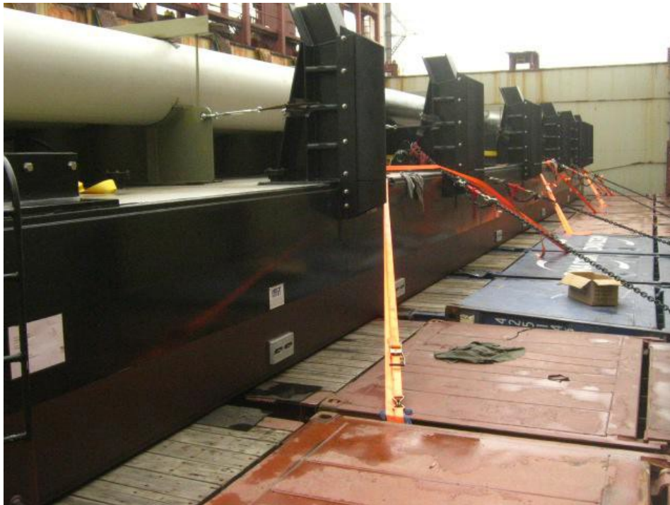
Cargo was properly stowed and secured under deck at bay 58
