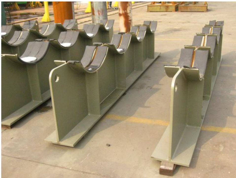
Steel cradles for pipes' placed
